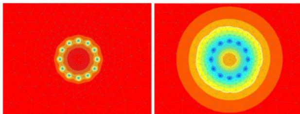
Artificial ground freezing, temperature distribution
