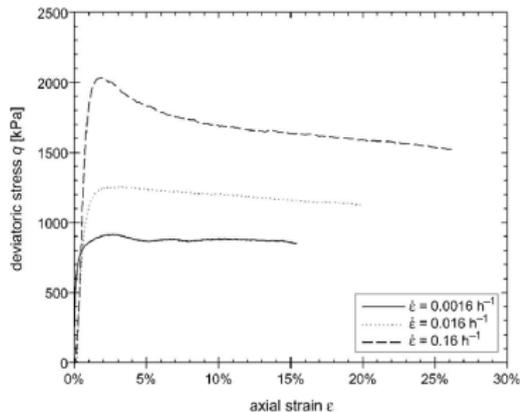
Stress-strain curves at different strain rates
