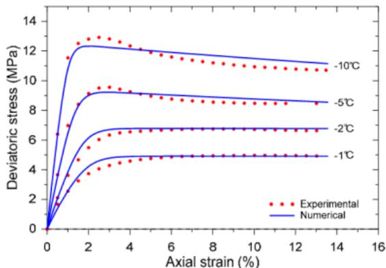
Stress-strain curves at different temperatures
