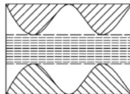
Schematic of ice increasing in an ice rich soil body
