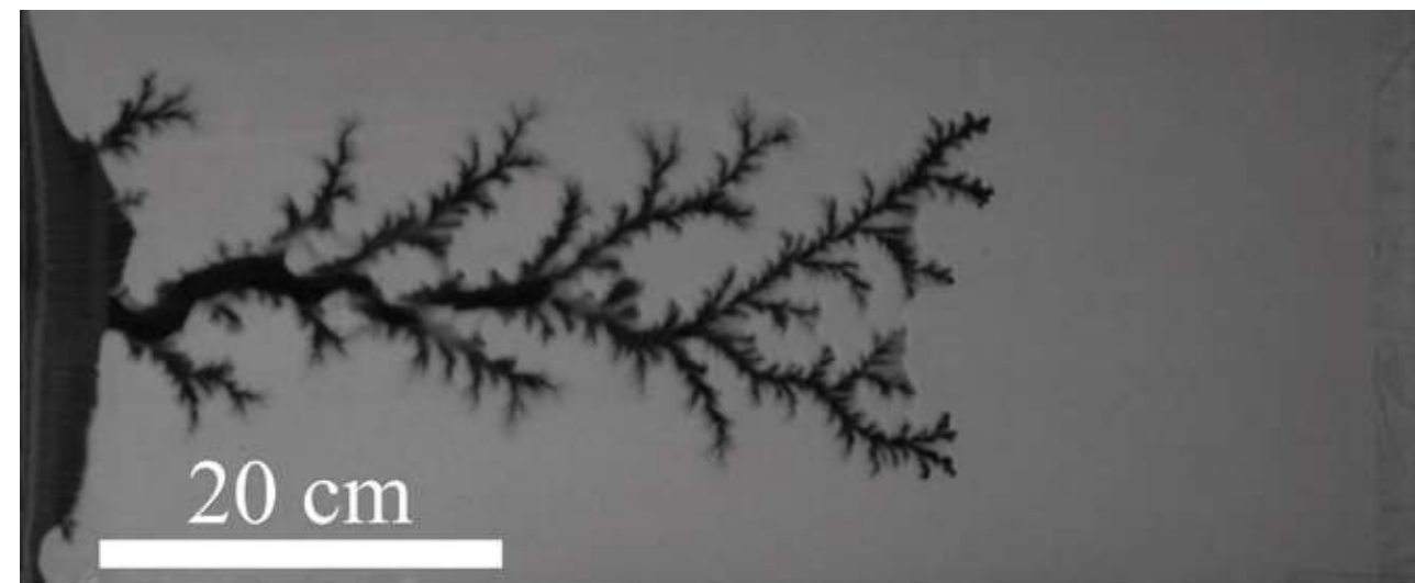
Fig. 1: A top-down image of the invasion channels (black) formed in a granular medium between two glass plates (gray) when air is injected from the left side at a constant pressure of 200 kPa. The long sides of the cell are completely sealed, while the right side has a filter which stops beads but allows air to escape. In this experiment, pressurized air forces its way from the left through the medium, leading to the formation of these branched channels.
