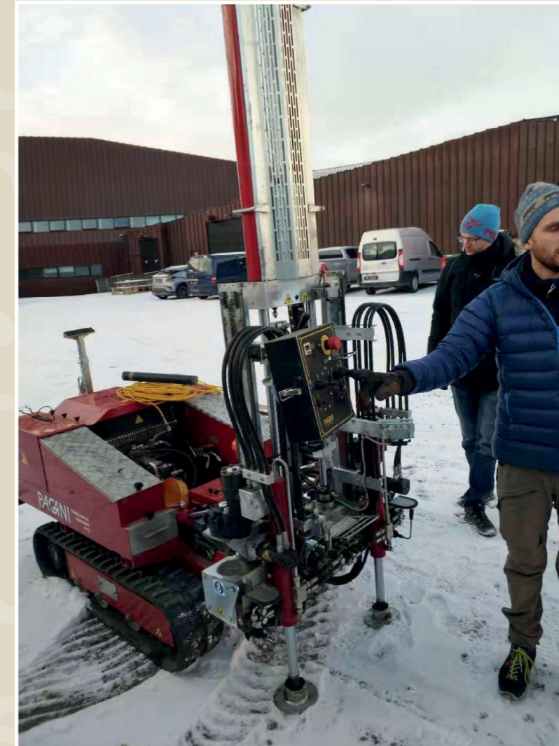
Figure 1. Field tests to measure pressures exerted by ice lenses that form inside partly frozen soils.
