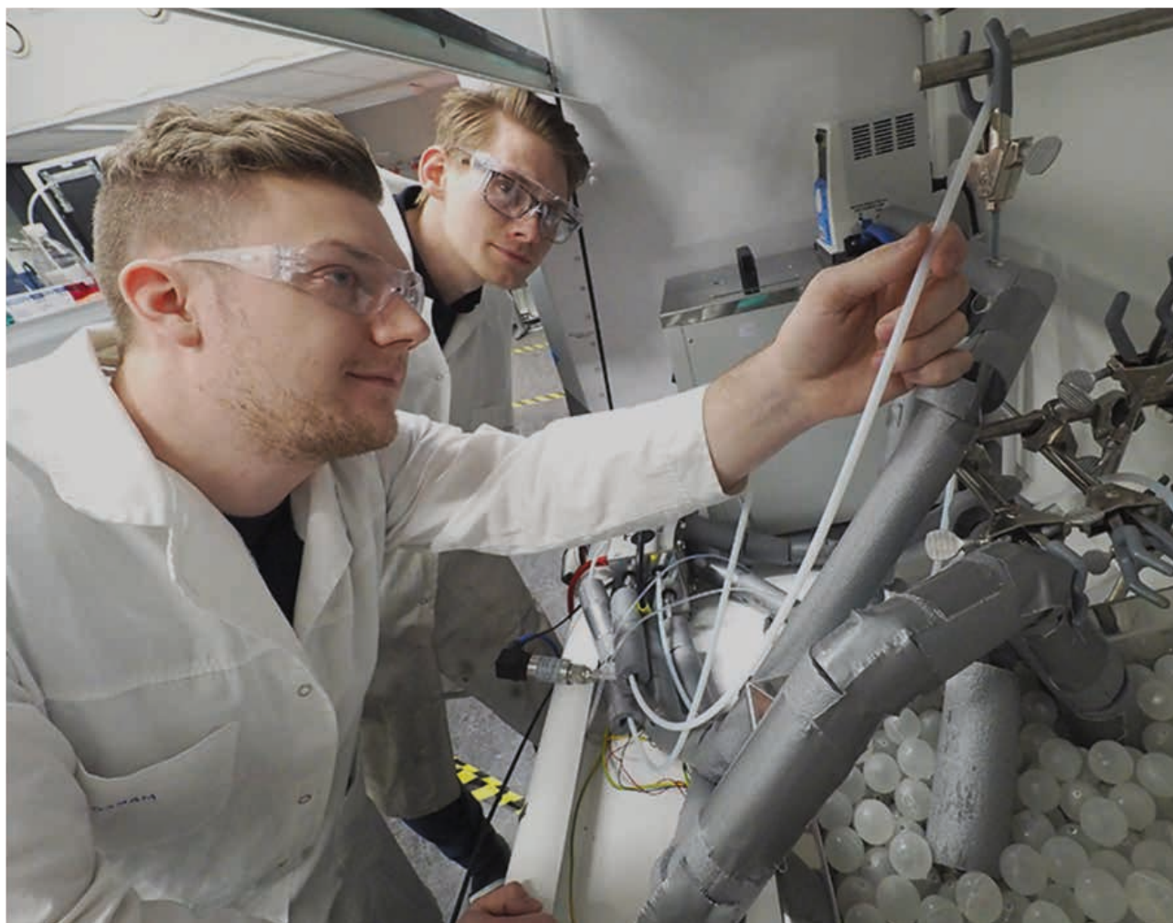
PhD candidates Marco Sauermoser and Olav Galteland are setting up a fuel cell test station in order to investigate new flow field plate designs. Photo: Per Henning
