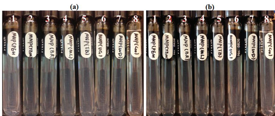
Figure 13. FNP-MD suspensions stability screening with different type of oils: (a), Day 1; (b), Day 30; (1: CO1; 2: CO2; 3: CO3; 4: CO4; 5: CO5; 6: CO6; 7: CO7; 8: Decane).
