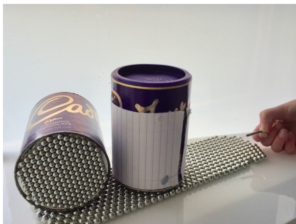
Figure 3: A home made set of patterned surfaces with low friction due to macroscale structural mismatch between the arrays of ball bearings. This device was built by second year undergraduate students in Dublin.
