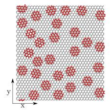
Figure 2: A top view of a simulation of a single layer of graphene flakes acting as a solid lubricant.
