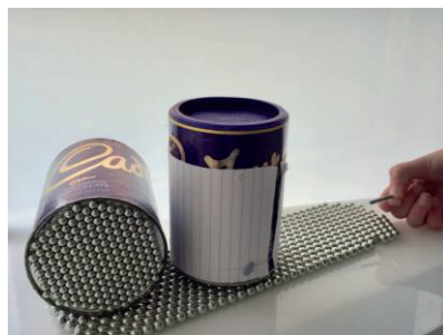
Figure: A homemade set of patterned surfaces with low friction due to macroscale structural mismatch between the arrays of ball bearings. This device was built by second year undergraduate students in Dublin.
