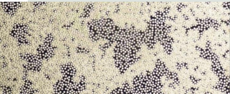
Figure: Detail of the trapped liquid clusters (blue) left behind after air (white) is slowly injected from the left in a quasi-2D porous network previously saturated with the liquid
